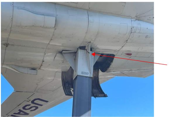
Photo 2: Exhibit from below on May 2, first visit - note the cracked gusset plate on the south side
